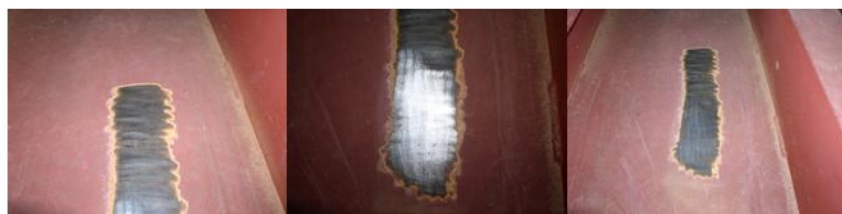
Close up of the stripped surface and profile created
